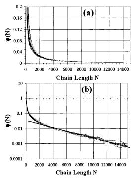
**Figure 8.** (a) Living MWD plotted on linear coordinates for the DNPMS/AIBN/MMA system for 11 samples, measured under comparable conditions. The MWDs are vertically shifted to compensate for their different normalizations. (b) MWDs in part a plotted on a semi-logarithmic scale. The straight line, a linear regression for chain lengths  $3000 < N < 16\,000$ , has slope  $-(2.8 \pm 0.4) \times 10^{-4}$ .
