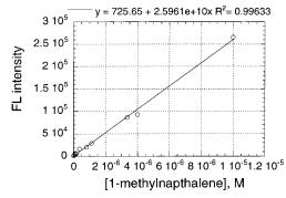
**Figure 13.** GPC FL detector integrated peak areas as a function of the concentration of the model label 1-methylnaphthalene in THF.
