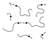
**Figure 1.** Schematic of a FRP mixture. Shaded background represents dead chains and monomer: at conversion  $\phi$ , this is a dead polymer solution at polymer volume fraction  $\phi$ . Living chains (foreground) are (i) growing at rate  $v_p$  monomer/s (proportional to propagation rate constant  $k_p$ ) and (ii) involved in interpolymeric reations which terminate growth, converting them to dead chains.
